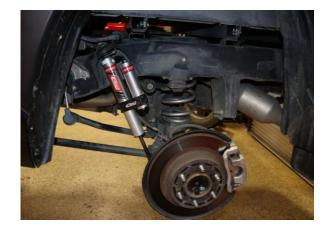
The reservoir should be mounted towards the top and pointing towards the back of the vehicle on both sides. Installing the reservoir shock without the alignment tab will result in shock damage and void warranty.
