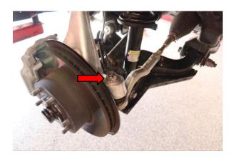
Step 4. Loosen but do not remove 24mm tie rod ball joint nut.
