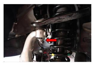
Step 7. Loosen, but do not remove the 19mm nut securing the spindle to the upper control arm.
