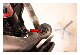
Step 20. Install outer tie rod ball joint into the spindle. Install 24mm nut onto the outer tie rod ball joint. Tighten to factory specification.
