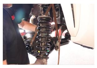
Step 13. Lower the shock assembly out down and out of the upper control arm and remove shock assembly from the truck.
