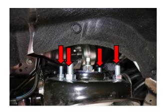
Step 17. Use a 14mm wrench to tighten four upper shock mounting nuts to factory specification.
