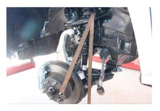
Step 9. Use a strap and secure the spindle to the frame to prevent damage to the axle CV joints.
