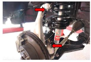
Step 22. Reinstall cotter OE cotter pin in upper ball joint and install new cotter pin in outer tie rod end ball joint.
