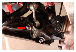
Step 19. Install 19mm bolt securing sway bar end link to the control arm. Tighten to factory specification.
