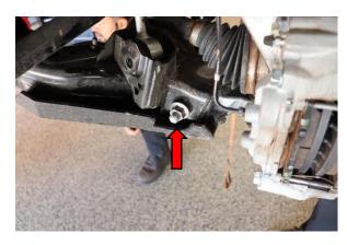
Step 11. Remove 22mm nut from lower shock mount bolt. Pull bolt from opposite side to remove.
