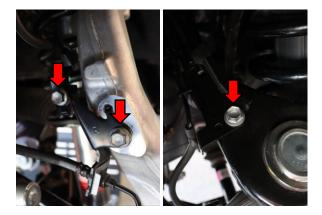
Step 21. Install three 12mm bolts securing the brake line and wheel speed wiring harness. Tighten to factory specification.
