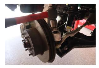
Step 5. Use a hammer to separate the tie rod ball joint from the spindle. Remove the 24mm tie rod ball joint nut. Remove the tie rod ball joint from the spindle.
