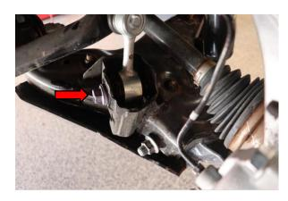
Step 6. Remove 19mm bolt securing the sway bar end link to the lower control arm.
