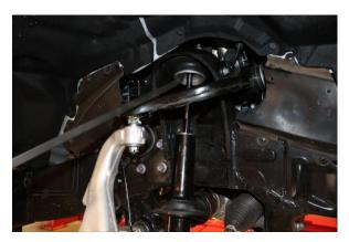
Step 10. Use a pry bar against the spring coils and the upper control arm to give the upper ball joint slack in the spindle. While holding pressure on upper control arm, remove 19mm upper ball joint. Slowly allow upper control arm to rotate up and away from spindle. Allow spindle to rest against installed strap.
