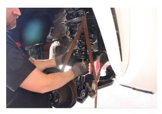
Step 12. Allow lower control arm to drop down slightly and rotate the bottom of the shock assembly toward the outside of the truck.
