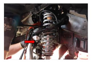
Step 18. Use a pry bar against upper control arm and spring coil to lower the upper control arm into the spindle. Install 19mm nut onto the ball joint finger tight and remove pry bar. Remove the strap supporting the spindle installed on step 9. Tighten 19mm upper ball joint nut to factory specification.
