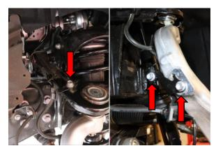
Step 3. Remove three 12mm bolts securing brake line and wheel speed sensor harness brackets.
