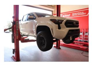
Step 1. Raise the vehicle on a suitable hoist and support it with the proper safety equipment. Use a 21mm socket to remove both front wheels. **Note:**Never work on or under a vehicle that is not supported by the proper safety equipment.
