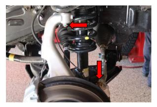
Step 2. Remove cotter pins from the castle nuts at the upper ball joint and tie rod ball joint.
