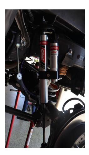
Reservoirs should be mount at the top and towards the rear of the vehicle as shown.
