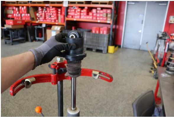
Step 9. Remove spring slider.
