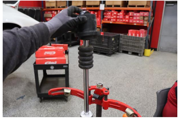
Step 14. Reinstall OE spring slider.
