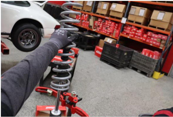
Step 15. Install Eibach main spring
