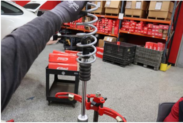
Step 13. Install Eibach secondary spring.
