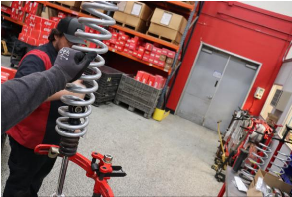
Step 15. Install Eibach main spring.
