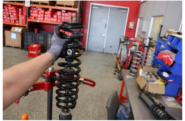
Step 8. Remove OE main spring.
