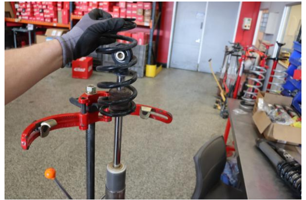
Step 10. Remove OE secondary spring.
