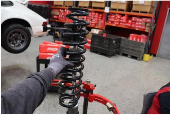
Step 7. Remove OE main spring
